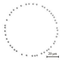
Image of colloidal particles trapped by a scanning laser beam to a circular optical trap,
