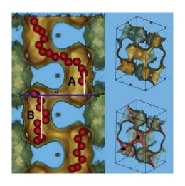
Schematic diagram of the diffusion of linear alkanes in Erionite (ERI), [D. Dubbledam *et al.*, PRL 90 245901 (2003) ]
